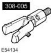
Axle oil seal remover 308-005 (LRT-37-004/2)
